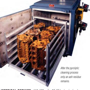
ELECTRICAL SERVICE: 110-125 volts, 50-60 hertz, single-phase, 5 ampere draw. Optional transformers available for other voltages.
